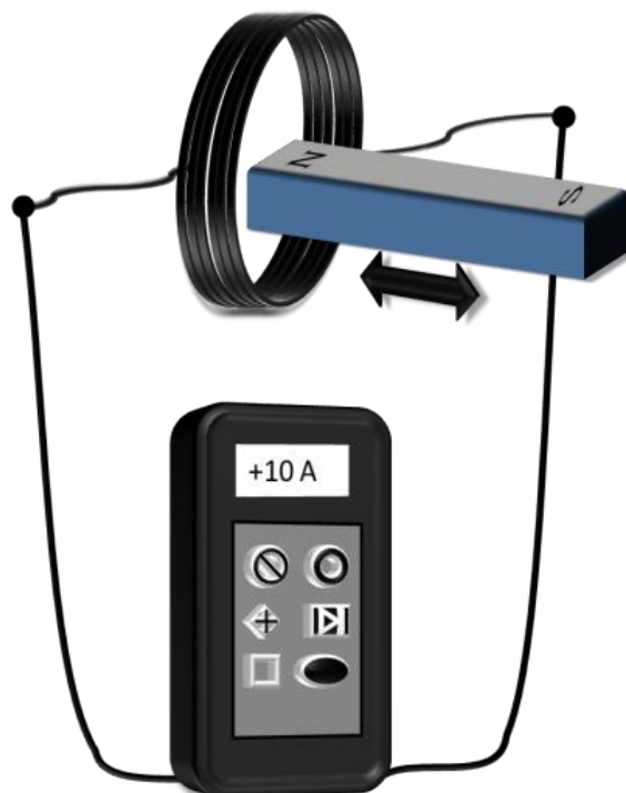
Figure 7: Illustration of the experimental setup of a modern variation of Faraday's experiment
