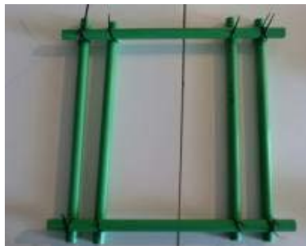
Figure 3. In this picture we can see how 6 pipes can be tied together in order to construct the frame of a platform. Note that this design is only a suggestion. Pupils should be encouraged to imagine and design their own ideas. This picture serves only as an example of how we can fasten the pipes together.
