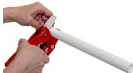
Figure 11. How to cut a PVC pipe
