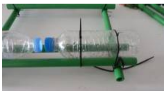
Figure 5. An example of how the bottles can be fastened on the frame using joined zip ties.
