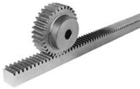
Figure 2. Using gears to transform motion
