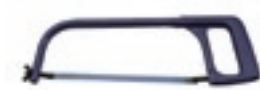
Hacksaw a saw with a narrow blade set in a frame, used for cutting metal
