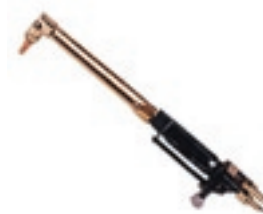
Cutting torch a device that uses fuel gases and oxygen to cut metals
