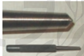
Centre punch a small steel tool with a conical tip used to punch a small indentation at the location of the centre of a hole to be drilled
